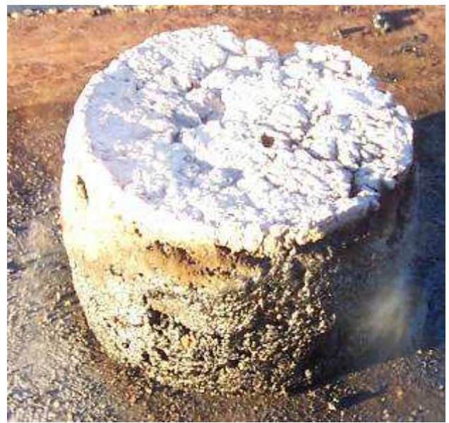
Coverfull Fireproof-System dopo combustione
